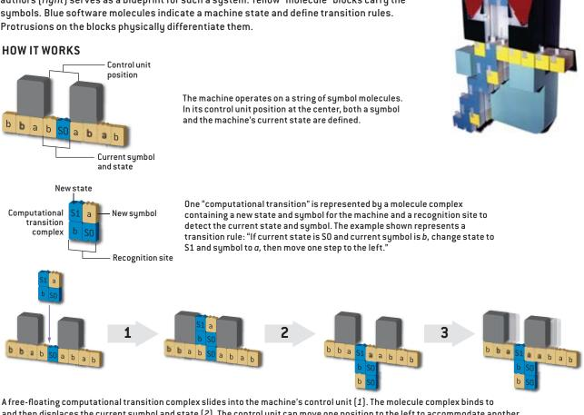
and then displaces the current symbol and state (2). The control unit can move one position to the left to accommodate another transition complex (3). The process repeats indefinitely with new states and symbols as long as transition rules apply.
